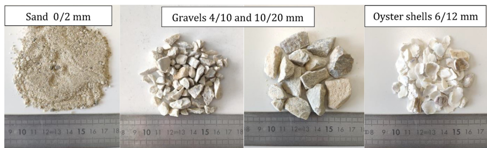
Fig. 2. The various types of aggregates used to elaborate the concretes of this study.
